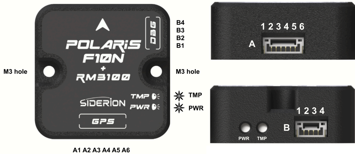
Figure 2. Polaris F10N pinout (top view & side views)
