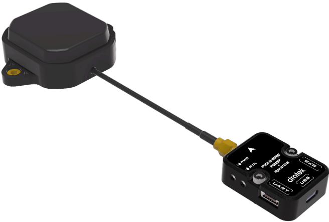
Figure 5. U-blox ANN-MB2 GNSS antenna attached to the Pioneer F20P
